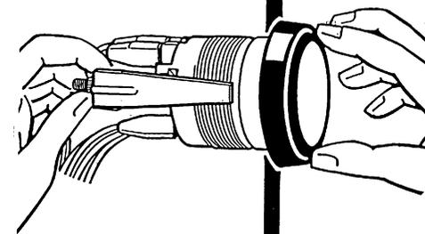
Caution: Window and bezel module to be cleaned with clear water only. Do not apply any chemicals
