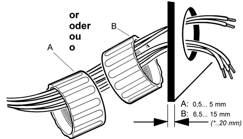
Install the display unit with the studs and the clamp (order no. N05 800 782) if exceptional stresses due to vibrations are to be expected at the point of installation (e.g. high-speed-boats).
