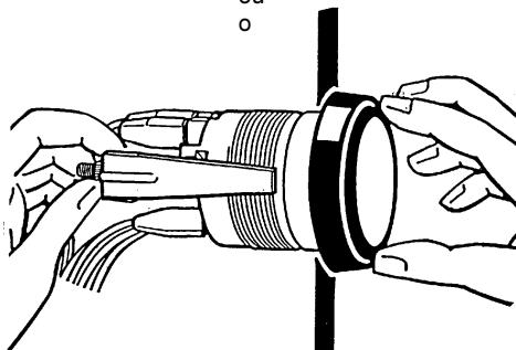
Slide the heat-shrinkable sleeve over the cable connections and then heat with a hot-air fan over the entire length until it shrinks. Always follow the safety advice of the hot-air fan manufacturer.
