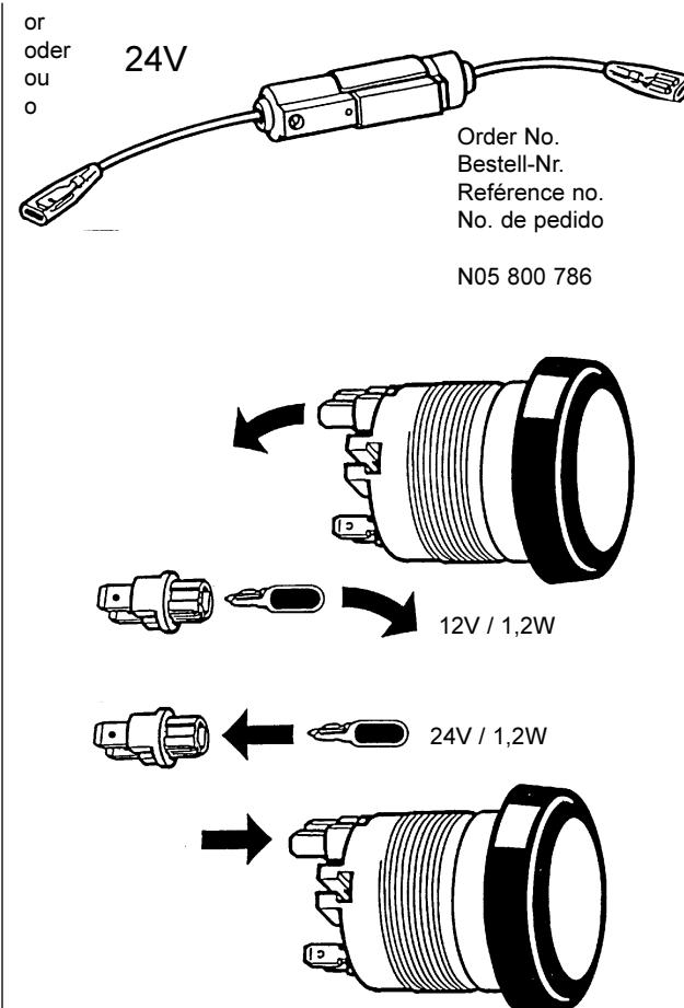
24V: Connect the series resistor (Rv) directly to the indicator unit.
