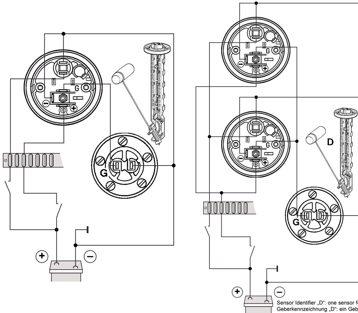
Sensor Identifier „D“: one sensor for two indicators
