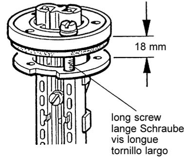
first insert long bolt with slot
