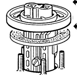
Fuel Tank Gauge (Lever Type Sender)
