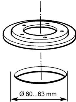
Tank flange for weld-mounting
