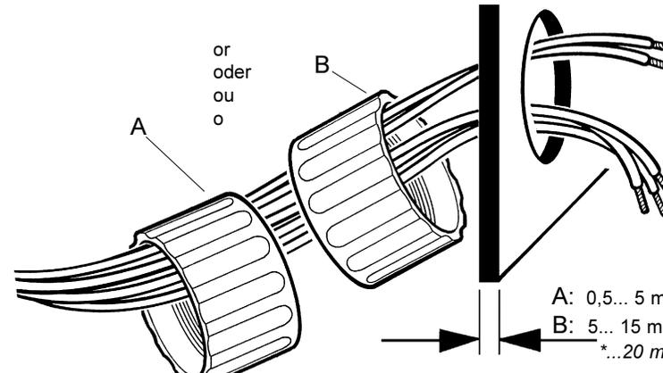
Install the display unit with the studs and the clamp (order no. N05 800 766 / \*N05 800 696) if exceptional stresses due to vibrations are to be expected at the point of installation (e.g. high-speed-boats).
