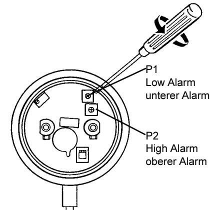
If the Low Alarm is not needed turn P1 clockwise to min.value (right end) carefully.
