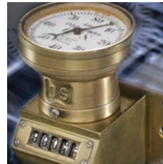
1902 – Eddy Current speedometer
