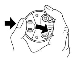
When changing lamp bulbs, carefully push the bulb out laterally with your thumb.
