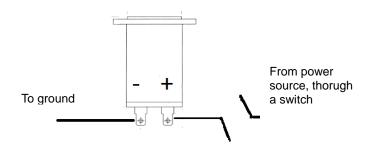
Switched power can be sourced from Igntion Switch, ignition system or other 'hot' source when engine is in operation.
