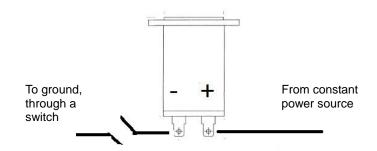
Switched ground can be in the form of a normally open pressure switch (that close when engine is running) or other ground source that is active only when engine is running.
