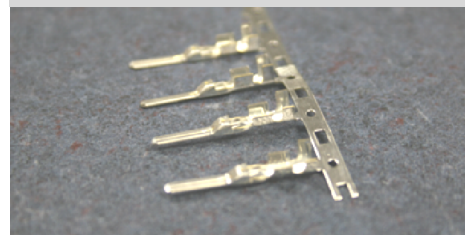
Connector pins for 10 pin harness to connect speedometer signal wire
