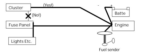
The diagram shows that there should not be a ground lead between the Cluster and the negative side (Common) side of the fuse panel.
