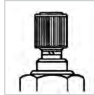
Connector 4 1 Pole common ground M4 stud or knurled nut
