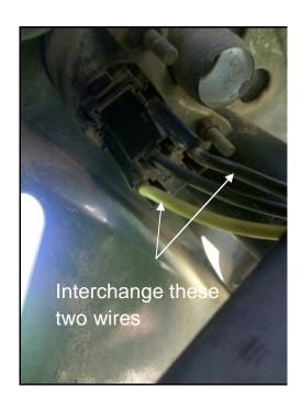
1) Power and Signal on gauge mating connector must be interchanged.
