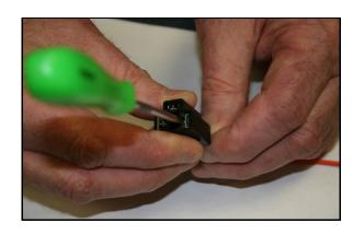
3) Pull on wires to release terminals from connector housing.
