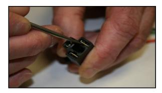
2) Using small pick or screwdriver in cavities next to terminals, push in to unlock terminals.
